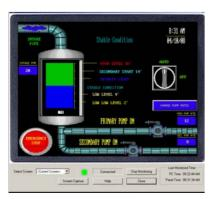
With UT-NVC software installed in your PC monitor could any screen on Touchpanel addressed by the software in Real-Time allowing system troubleshooting and/or management review of the machine opertaion.
